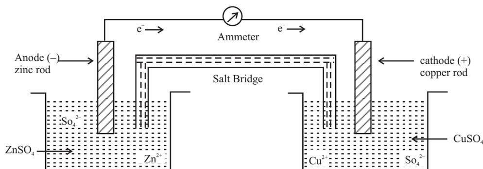
Fig. 13.6 : Daniell cell having zinc and copper electrodes
