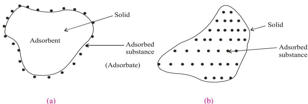
Fig. 15.2 : (a) Adsorption (b) Absorption
